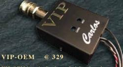
VIP-OEM is a single-channel pickup based on a CP-1A VIP circuit and VIP-Double look, incl. 2 mini pots (middle + gain) and a soundhole gain pot. It has been used in diverse limited productions as of Furch and Breedlove guitars. Comes with a undersaddle coaxial transducer.
